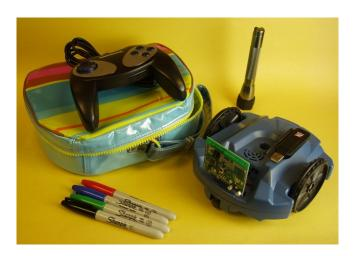
Figure 1: The IPRE Robot Kit, Fall 2007. Clockwise, from top-left: lunchbox carrying case, gamepad, flashlight, Scribbler robot with IPRE Fluke (camera and serial Bluetooth adaptor), USB Bluetooth dongle (for computer if it doesn't have Bluetooth), and drawing pens.
