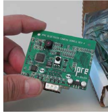
The Fluke Dongle adds Bluetooth and other capabilities to the Scribbler.
