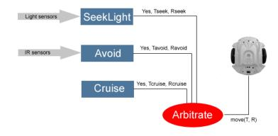
In the diagram above, we have shown the three basic behaviors that we are trying to combine: Cruise, Avoid, SeekLight. Each of these behaviors outputs a triple: Yes/No, Translate Speed, Rotate Speed. A Yes implies that the behavior module has a recommendation. No implies that it doesn't. That is, it
