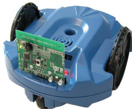
The Scribbler robot with the Fluke Dongle.
