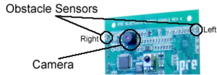
The values reported by these sensors range from 0 to 7000. A 0 implies there is nothing in front of the sensor where as a high number implies the presence of an object. The sensors on the sides can be used to detect the presence (or absence of walls on the sides).
