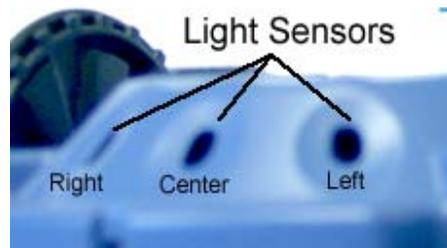
The values being reported by these sensors can be in the range [0..5000] where low values imply bright light and high values imply darkness. The above values were taken in ambient light with one finger completely covering the center sensor. Thus, the darker it is, the higher the value reported. In a way, you could even call it a darkness sensor. Later, we will see how we can easily transform these values in many different ways to affect robot behaviors.
