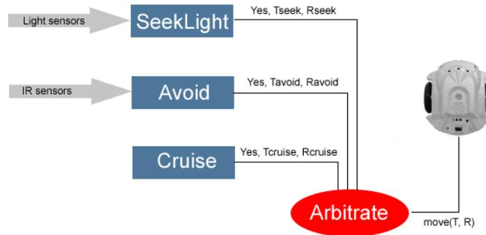
In the diagram above, we have shown the three basic behaviors that we are trying to combine: *Cruise*, *Avoid*, *SeekLight*. Each of these behaviors outputs a triple: *Yes/No*, *Translate Speed*, *Rotate Speed*. A *Yes* implies that the behavior module has a recommendation. *No* implies that it doesn't. That is, it
