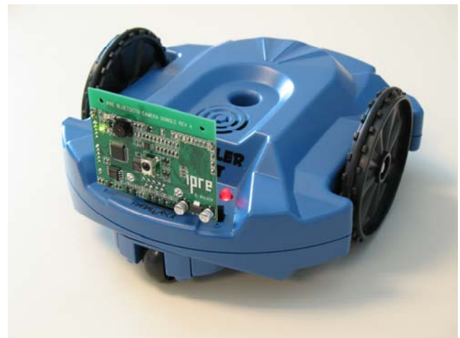
Figure 2. The Scribbler Robot with IPRE Fluke Board
